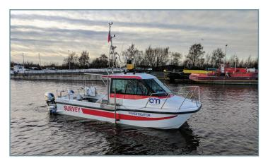
Multibeam echo sounders provide significant advantages over traditional survey. Surveying the bed with a wide band of narrow acoustic beams means it is possible to obtain complete coverage of the bed topography, allowing surveys to be completed faster and minimising risks such as weather delay.
