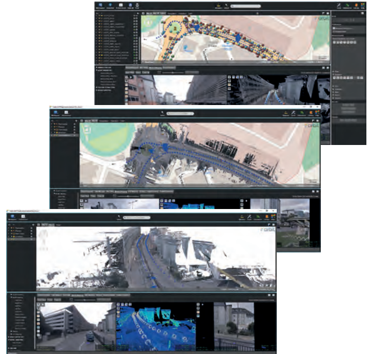
Orbit GT software supports all 3D mapping data and has products to manage, extract, process and share. The screenshots above are from a highways mapping project and show the 360-degree imagery and point cloud data within Orbit's 3DM Feature Extraction software.
