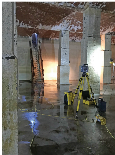
Figure 1: Trimble SX10 Laser Scanning of Reservoir
