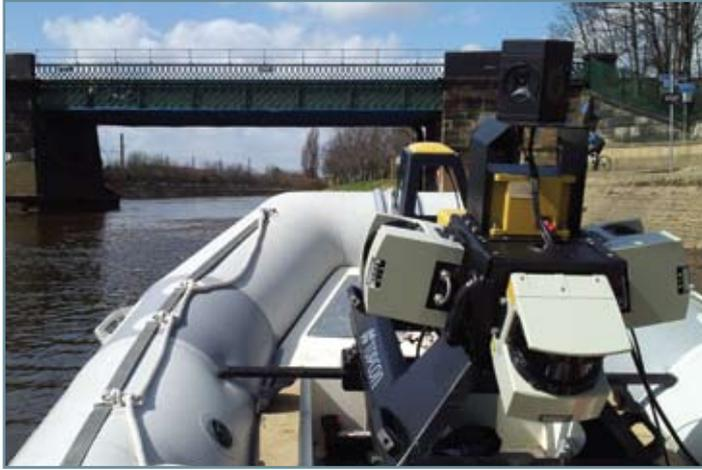
3D laser scanning systems may be deployed from the bridge, adjacent banks and even pier structures to provide the highest resolution and highest order accuracy 3D LiDAR models.
