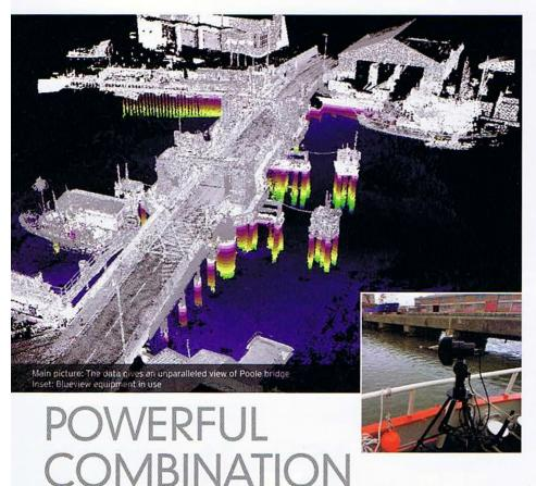
Above and below-water surveys of an existing bridge have been combined to create a very detailed model for use in planning repairs
