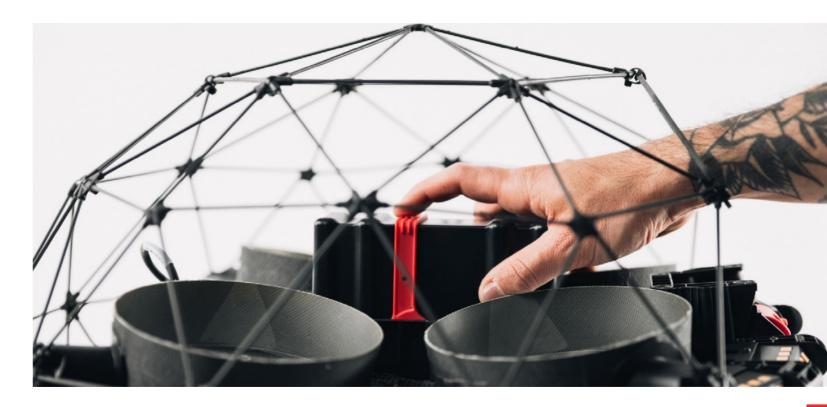
New insert and lock mechanism to ease battery manipulations
